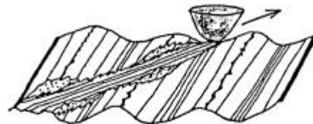
(c) Added AE surface of the ductile-mode grinding
